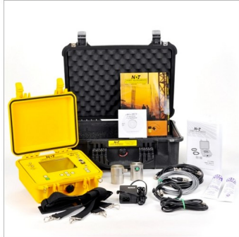
V-Meter MK IV™ Ultrasonic Pulse Velocity System
